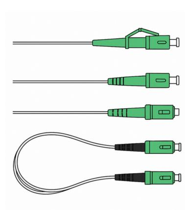
Pigtails feature a pre-terminated connector on one end and an open fiber end for fusion splicing to primary coated fibers.
